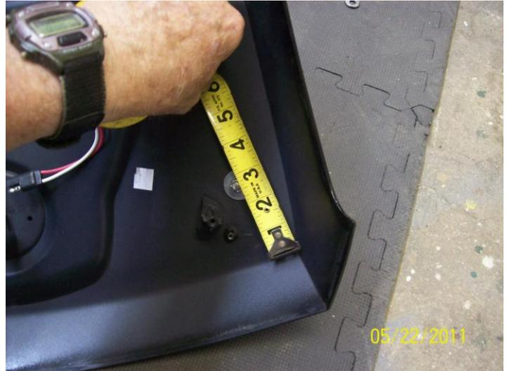
Upper-shorter-or front leg drilling positions.  $\frac{1}{2}$ " from side bend and  $1\frac{1}{2}$ " from pocket bend.
